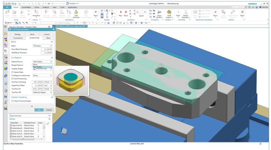
**5-axis milling** – CAM Pro offers highly flexible 5-axis programming functions combining highly automated elements for tedious tasks such as geometry selection and detailed user control for roughing and precise machining. 5-Axis Roughing allows for greater efficiency and longer tool life when machining complex geometry
