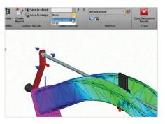
If you don't get your desired results the first time – such as if our beam from the previous example has a displacement of more than 1 mm – Solid Edge synchronous technology allows you to easily make changes to your design depending on your objectives. However, rather than manually making time-consuming changes to reach the appropriate results, Solid Edge provides simulation optimization to automate and optimize your design.
