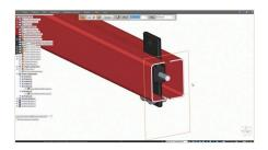
To optimize the simulation analysis, you can represent sheet metal end caps as surfaces, a much more lightweight representation for the study. Mixing surface and general body meshes is a great way to simulate sheet metal bodies along with formed parts.
