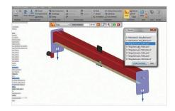
Once everything is set up, you can mesh and solve the study. Solid Edge gives users complete control over the mesh settings for both solid and surface meshes. You can easily change your view of results; for example, from stress distribution to displacement using a dropdown.
