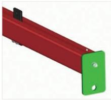
With the end caps defined, you can then set up the study. No matter the type of study being run, common steps are used to set them up. You have geometry, loads and constraints – just like in beam analysis – but in the assembly study you need to define how the parts connect (this was done automatically in the beam analysis based on the proximity of the beams to one another).
