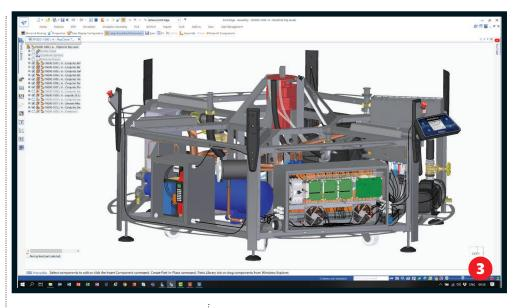
to components/subsystems and quickly pick points and geometric features/surfaces to snap them to along the way. It'll save you all of the effort of positioning clips and other mounting components you'd typically have to organise and give you solid, sufficiently accurate data on wire lengths, which subsequently get passed back to the BOM.
